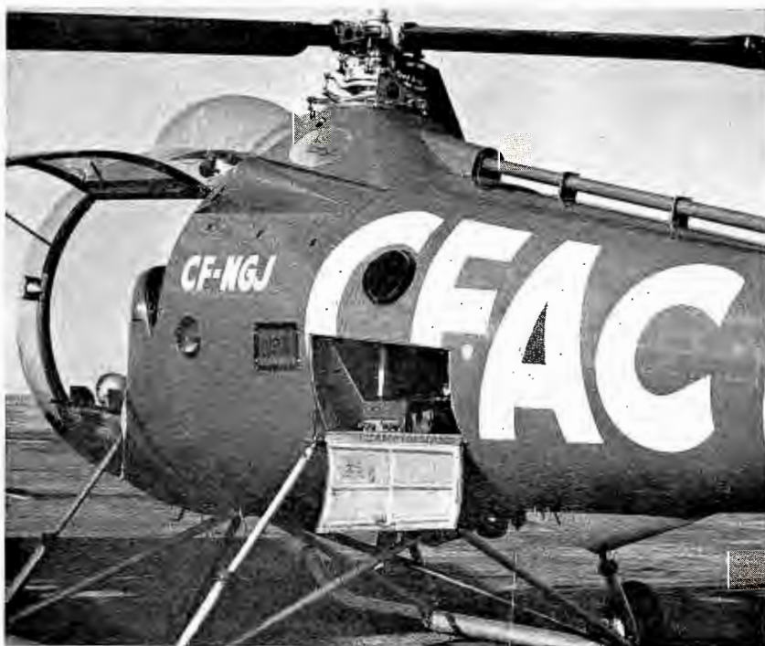
Fig. 1. Brantley B2 helicopter showing location of the equipment for remote use.
